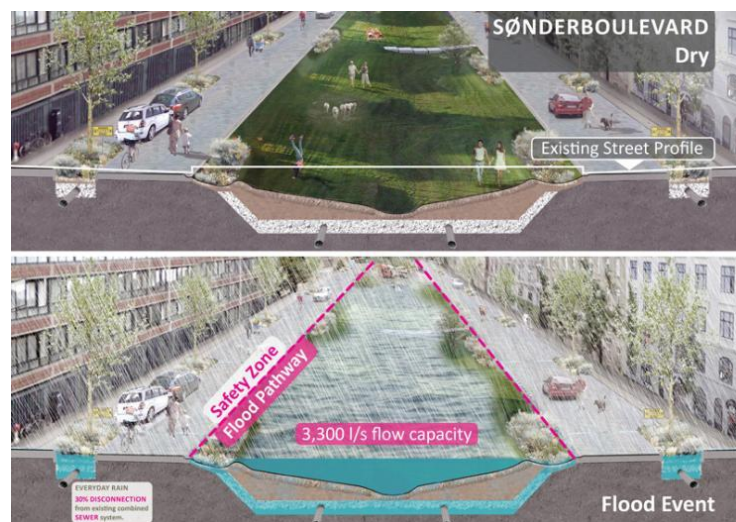
Fig 3. Copenhagen Cloudburst project for urban resilience using GI for managing flood risk (Sources: www.ramboll.com)
