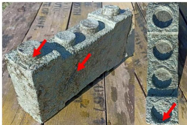
Gambar 15. Prototipe bata lego sampah plastik jenis polimer *High-density Polyethylene* (HDPE)
